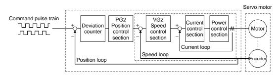
A general servo system configuration is shown above. The servo control system consists of three loops: current loop, speed loop and position loop. Among these three loops, the response of the inside loop must be increased 4 to 6 times higher. If this condition is not satisfied, vibration will be generated. If the condition further worsens, hunting will occur.
